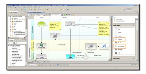
I want to point out a couple of shapes that can be used in complex process diagrams like this one. The **AND** gateway allows you to define multiple paths that execute in parallel, and that can all come together again when they've all completed. The **XOR** join shape allows you to specify that only one of multiple paths completes before the process continues. These types of paths are possible because a BizLogic process can have multiple tasks going on at the same time.
