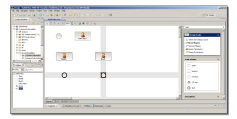
Now I need to connect all these shapes together in the sequence they should follow. The default when you select **Connect Shapes** is the same as for a regular process. You draw arrows between shapes to establish a sequence. The Start step just links directly to the Data Input step. That step in turn can go either to the BuildIt Activity or to the BuyIt Activity. The process doesn't do anything else, so BuildIt just goes to an End step, and so does BuyIt. Here all the links are complete:
